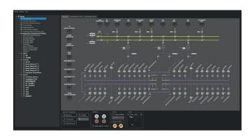
The ARKENS Studio configurator enables all SCLE system equipment, protection relays, unit computers, operator stations and remote control gateways to be configured via a single software tool.
